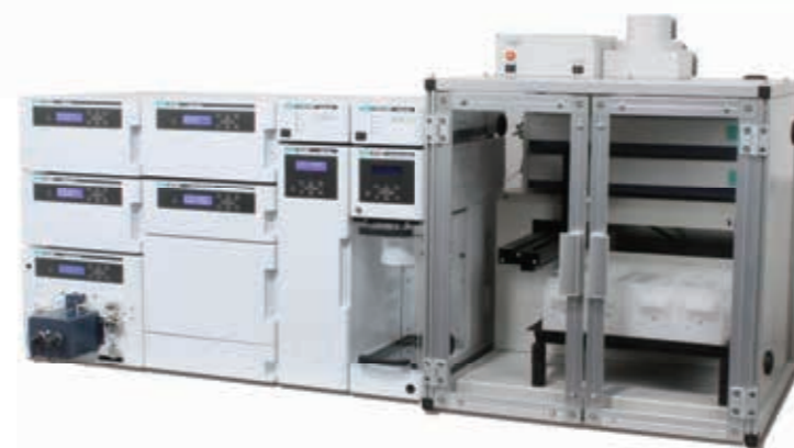
System configuration example of Semi-Prep SFC System
